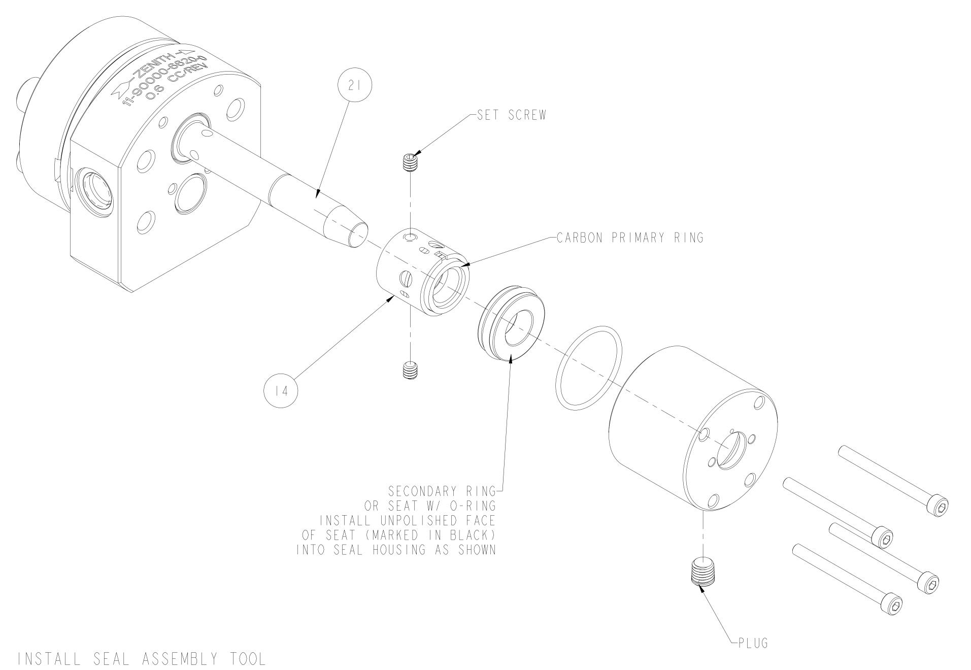
ONTO SHAFT TO COVER KEYWAY DURING SEAL INSTALLATION, TO PREVENT DAMAGE.
