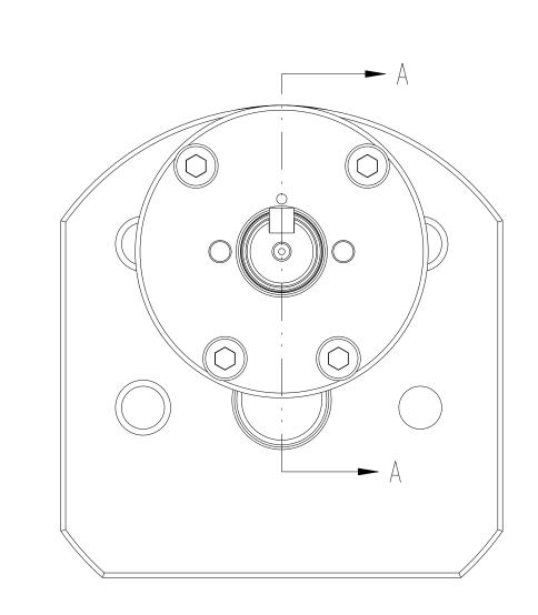
LUBRICATE UNDERSIDE OF CAP & THREADS ON FASTENERS WITH ANTI-SEIZE COMPOUND PRIOR TO ASSEMBLY.
